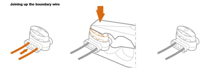
Landroid box includes two small, waterproof boundary wire connectors. They can be used for the following:
